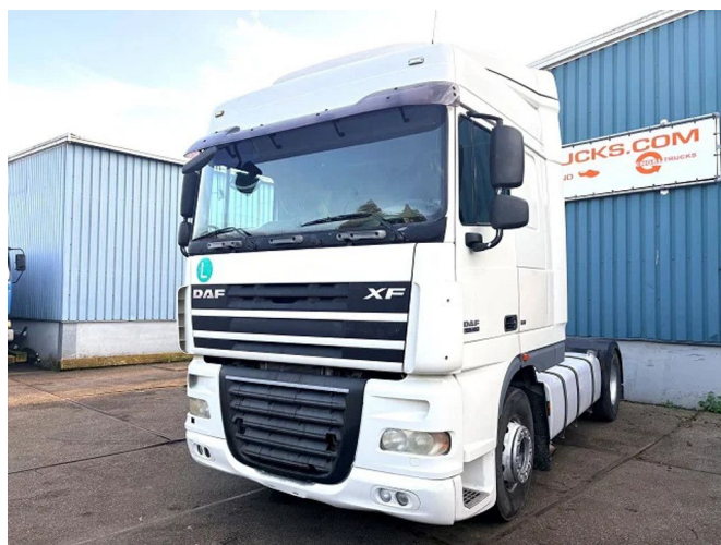
DAF XF 105.460 SPACECAB (ZF16 MANUAL GEARBOX / EURO 5 / 2x DIESEL TANK / AIRCONDITIONING / MX-BRAKE / ETC.) 4x2
